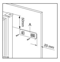
Fix cover (C) on guide (A) until it clips into place.
